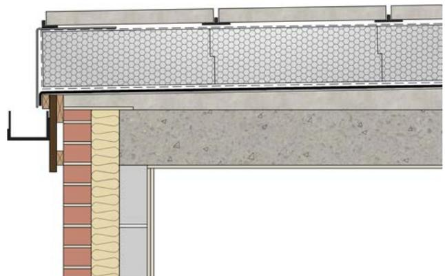
Figure 7. Ballasted inverted roof – detail at eaves
