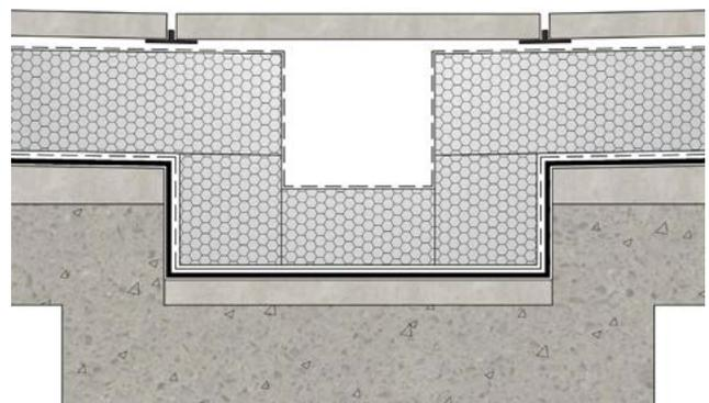
Figure 6. Ballasted inverted roof - insulation over internal gutter
