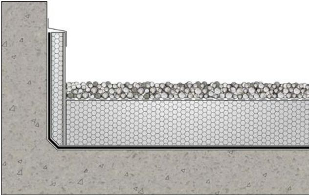
Figure 3. Inverted roof – detail at upstand
